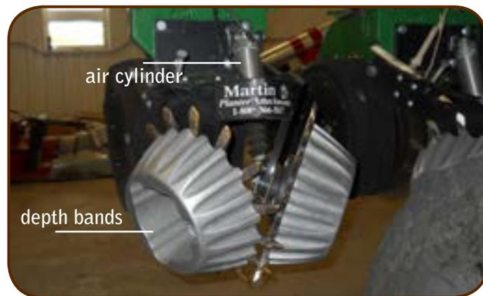
A close-up photo of the new trash wheels on the planter. Notice the depth bands for depth control and the air cylinder for adjustable down force.
