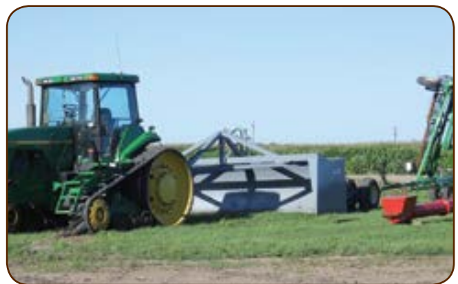
The John Deere 8400T and box scraper help to level our tile lines.
