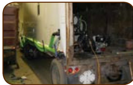
Plumbing was upgraded on the water truck from two to three inches to make filling the sprayer quicker.
